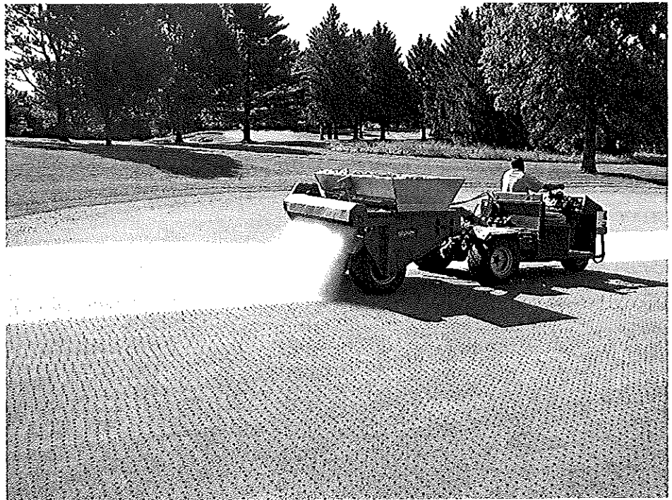
A heavy topdressing application allows aeration holes to be filled completely and limits the need for excessive dragging. This application completely fills the aeration holes to maximize the benefit of the aeration practice and limit disruption to playability. Completely filled holes also provide a uniform appearance on the putting green, which can affect perception of green smoothness as healing progresses.
